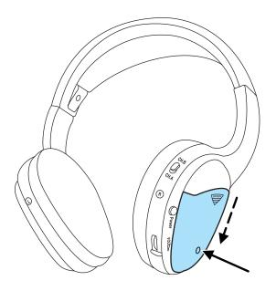
To install the batteries, remove the screw at the bottom of the cover. Then, lightly press down on top and slide the cover off.
